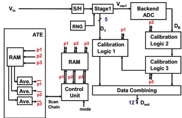
Fig. 6. Block diagram of the pipelined ADC with background calibration logic in [13], plus our proposed on-chip test-assist logic.
