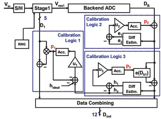
Fig. 4. Block diagram of the pipelined ADC with background calibration logic in [13].
