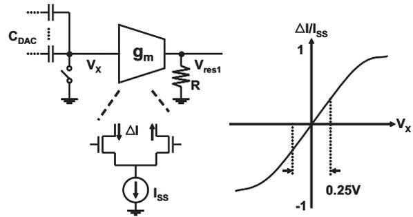
Fig. 5. Open-loop residue amplifier with nonlinearity used at the end of "Stage 1" in Fig.4.
