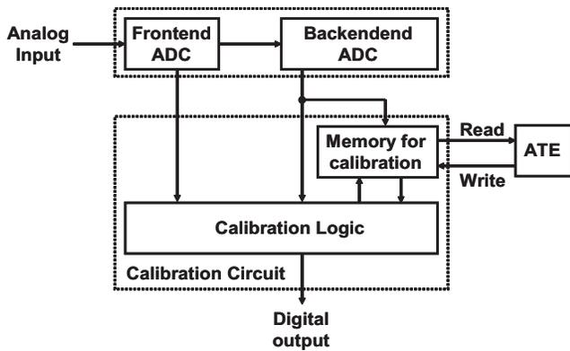
Fig. 2. Block diagram of a typical pipelined ADC with background calibration and memory read/write circuit.
