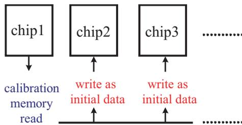
Fig. 3. Explanation of the proposed method for fast calibration convergence. The ATE reads the converged data from chip 1 memory and downloads it to chip 2, 3, 4, ... as initial data.
