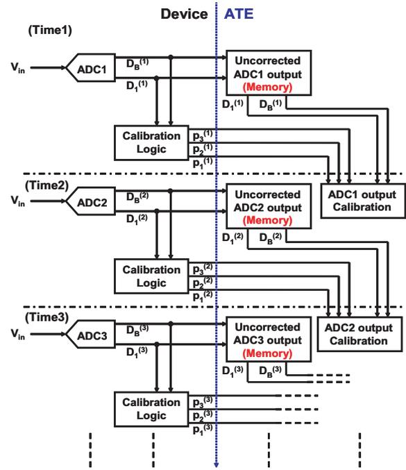
Fig. 9. Proposed method where the calibration and function test are performed in pipelined manner.
