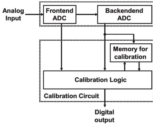
Fig. 1. Block diagram of a typical pipelined ADC with background calibration.
